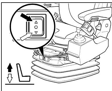
Press the rocker switch at the top or at the bottom to move the seat upwards or downwards. If adjustment reaches the top or bottom end stop, the height will be adjusted automatically, so as to ensure a minimum spring travel.
